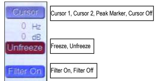
**Freeze Button:** To aid in setting the cursors and making measurements, pressing this button causes the waveform to freeze.
