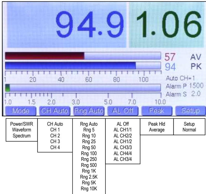
The above picture shows the Power/SWR mode, with menu choices listed below each button. The last choice in each list wraps around to the top.
