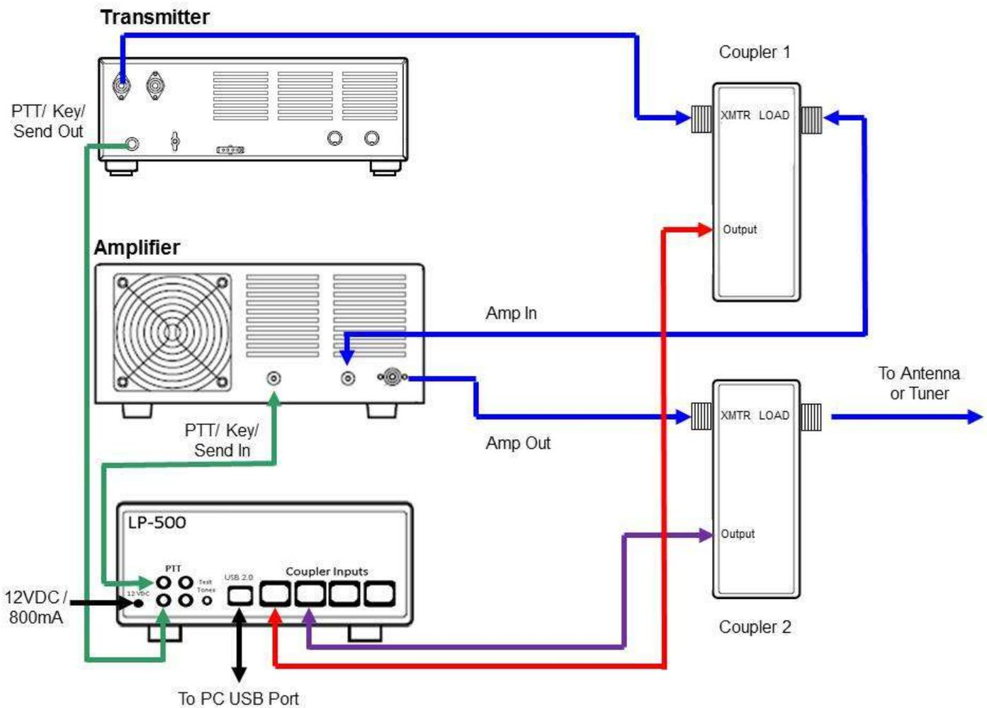
Fig.1. Shows installation with two couplers and PTT Alarm connections. The use of two couplers allows viewing of amplifier linearity with a trapezoidal display. PTT Alarm connections are optional and designed mainly for older amplifiers with no built in protection.
